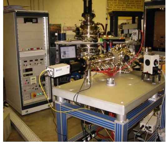
Fig. 1 PEEM Imaging column with magnetic lenses. Resolution: 8 nm (Hg arc lamp); Field of view: 2 - 175 \mu\text{m} , base pressure: < 2 \times 10^{-10} Torr; Sample temperature: 100 to 2200 K.
