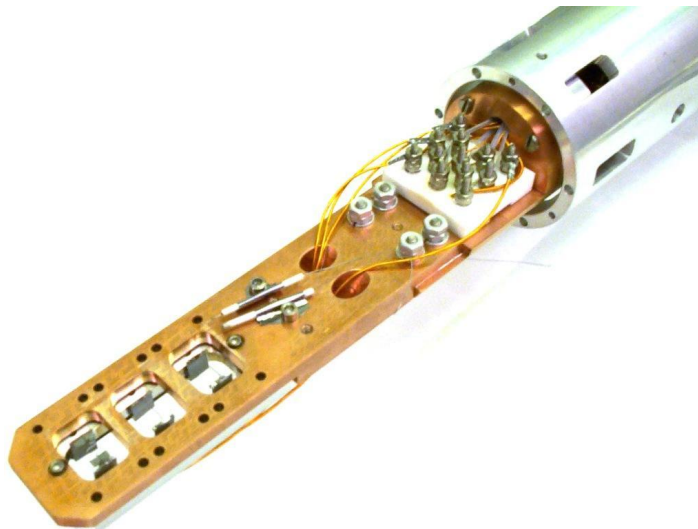
Figure 8. E-Beam Heating Sample Holder.
