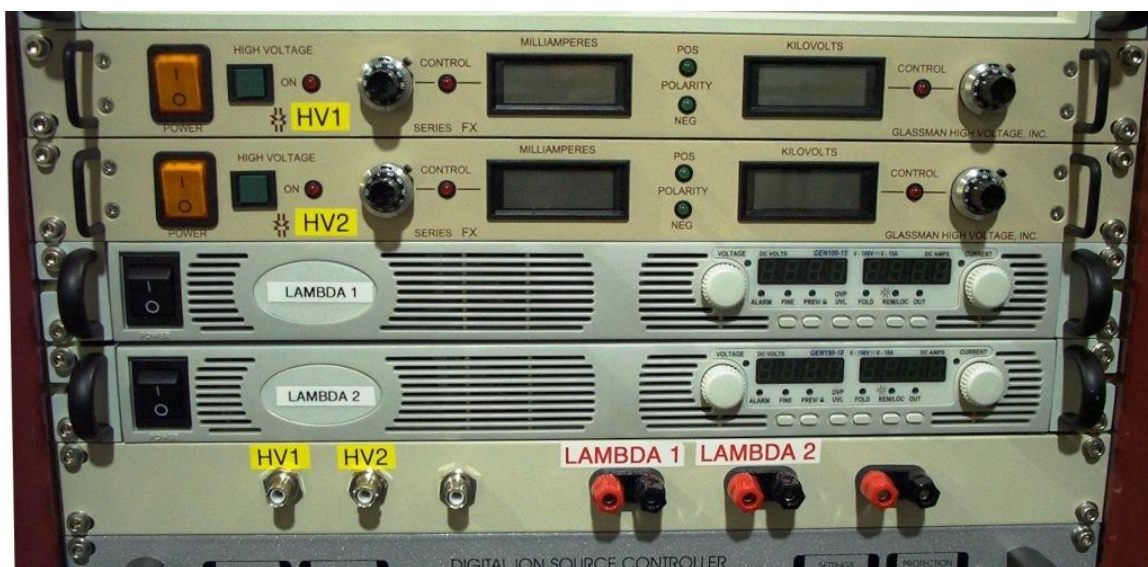
Figure 7. High Voltage and Current Supplies.
